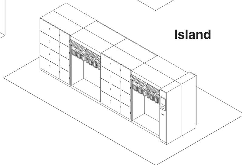
Here some examples to illustrate the installation variants that checkSpot offers. The number and arrangement of the different modules can be adapted to any needs and spatial conditions and thus be combined to a customized system. A complete system requires at least one terminal.
