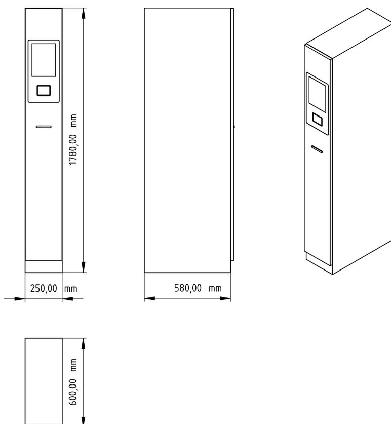
Connection for power supply (100-240V / 50-60 Hz), network (optional) and the modules to be managed on the backside.
